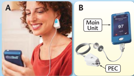
Figure 1: [A] Conducting a glucose measurement; [B] GlucoTrack contains a Personal Ear Clip (PEC) and a Main Unit (MU).
